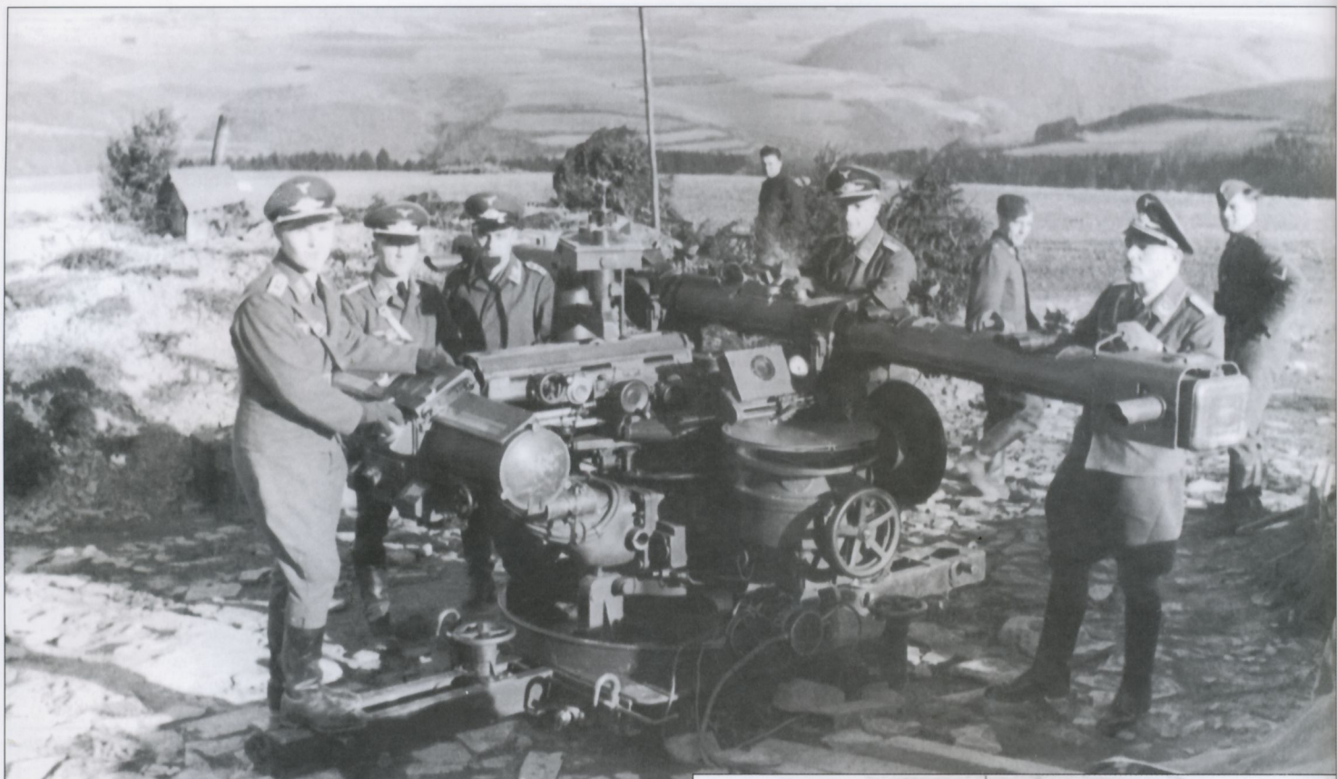
Two photos of officers, NCOs (center and far left) standing around a Kommandogerät 36 as junior enlisted men look on from a distance. This device, a state-of-the-art computer for its time, took a target's height and range plus its azimuth and angle of slant to compute its rate of change and most importantly, compute the enemy's predicted future location.
