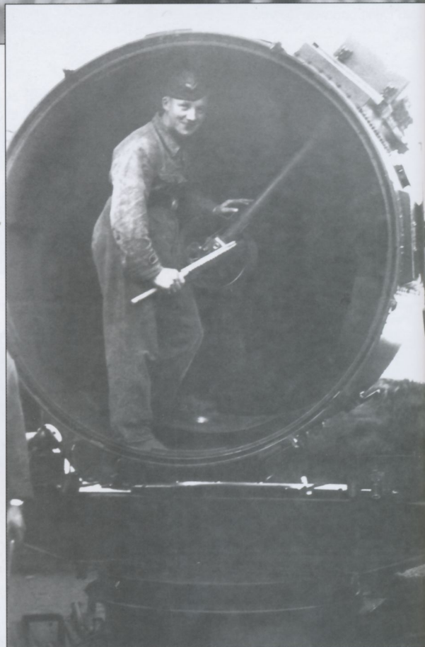
Crew of 60cm searchlight used with medium and light flak. One man wears blue-gray twill coveralls while other is in Drillichanzug . In good weather the 135 million candlepower light could throw a beam 5,000 feet vertically.
