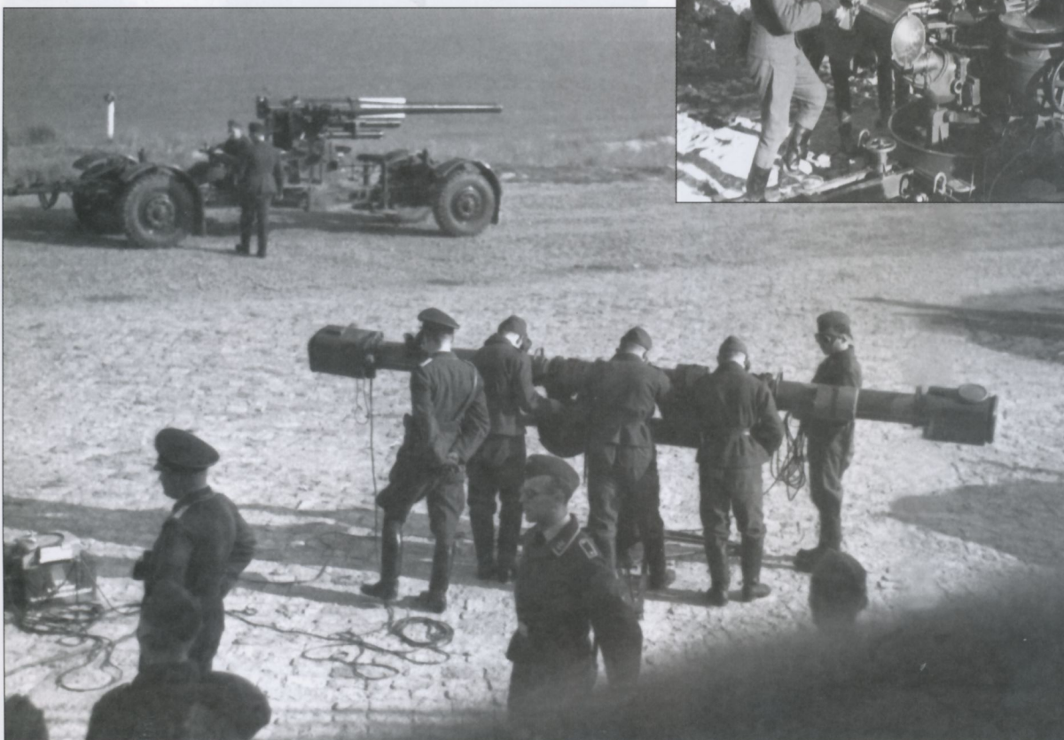
Crew puts standard 3m rangefinder into operation. Two officers (left in Schirmmütze ) and a Feldwebel (center) are in attendance. Rangefinders and searchlights were often used in conjunction with trumpet-shaped sound locators (complete with "lag calculators") to get an accurate fix on enemy aircraft.
