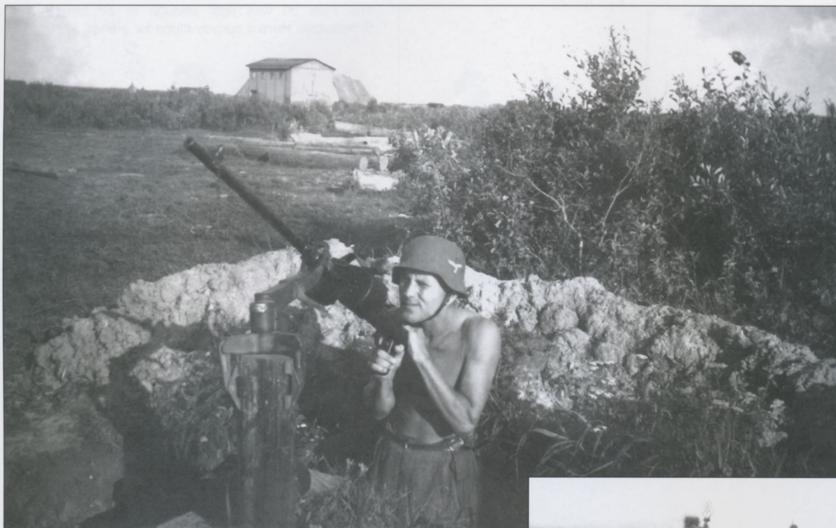
Two photos of the standard Luftwaffe aircraft machine gun, the 7.92mm MG15, mounted for ground use. Both use the Doppeltrommel (double drum) that could hold up to 75 rounds. As the Luftwaffe aircraft loses mounted guns like these were no longer need in flying units.
