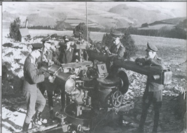
Two photos of officers, NCOs (center and far left) standing around a Kommandogerät 36 as junior enlisted men look on from a distance. This device, a state-of-the-art computer for its time, took a target's height and range plus its azimuth and angle of slant to compute its rate of change and most importantly, compute the enemy's predicted future location.
