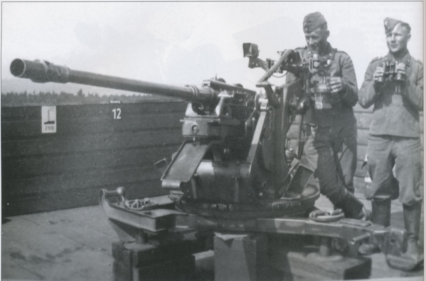
A Flak 30 here manned by two men in Fliegerbluse and Feldmütze (also known as Fliegermütze ). Small sign on wall to left indicates there is a smokestack at 2500 mils. Of the 2cm (.79 inch) family of weapons, Models 28/29 were developed by Oerlikon for the Kriegsmarine, Model 30 by Rheinmetall-Borsig and the Model 38 by Mauser.
