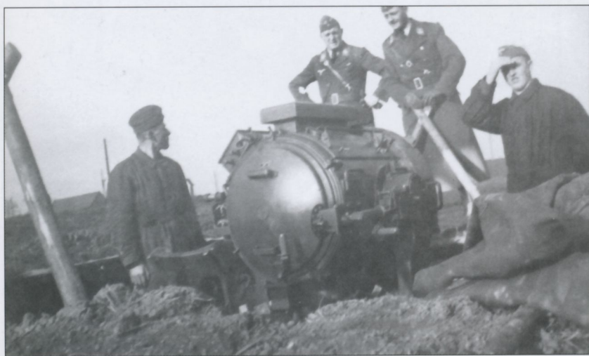
Two officers inspect dug-in 60cm (24 inch) searchlight and crew. Not counting the vehicle driver this light had a crew of four and was powered by an 8kw generator.
