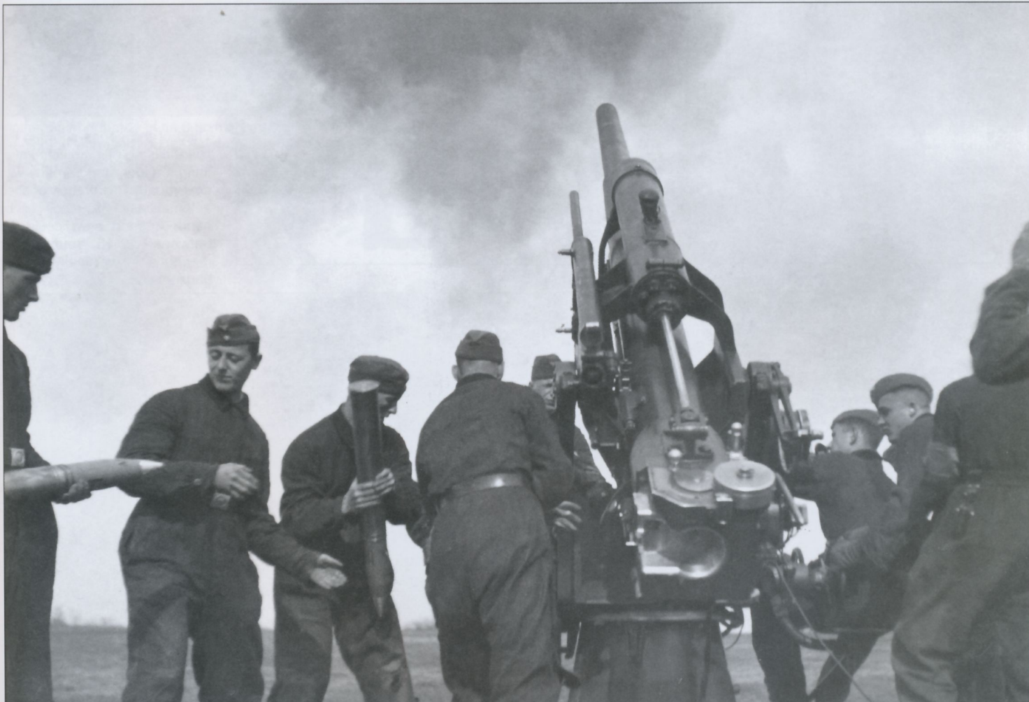
Men in black coveralls go through live-fire crew drill. This 8.8cm is at full 1m recoil. Men called "ammunition numbers" to immediate left of gun with shells up-side-down are setting tip of round in device next to the breech that will set automatically altitude of burst.
